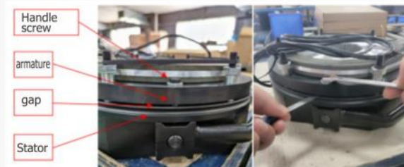
Handle clearance, on both sides of the brake
