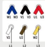
Wiring bridge installation for YY/Y connection (9 lead wires).
