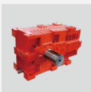
JRHD Bucket Elevator Gear Units Size: 5-16 Ratio: 25-71 Input power: 21.8-1775HP Output torque: 97284-1530012 lb-in
